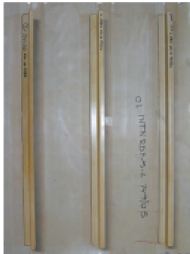
Fiber Metal laminate delamination/debond
